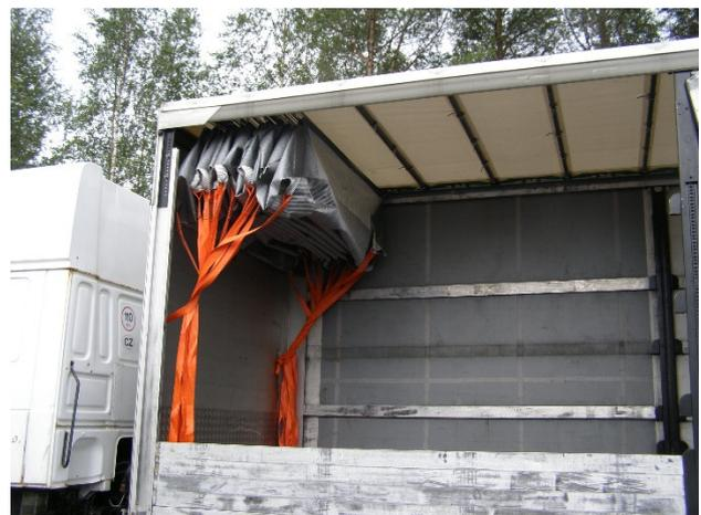
not in use FIX Road® can easily be stored against one end of the vehicle. Space requirement is only 60cm.
