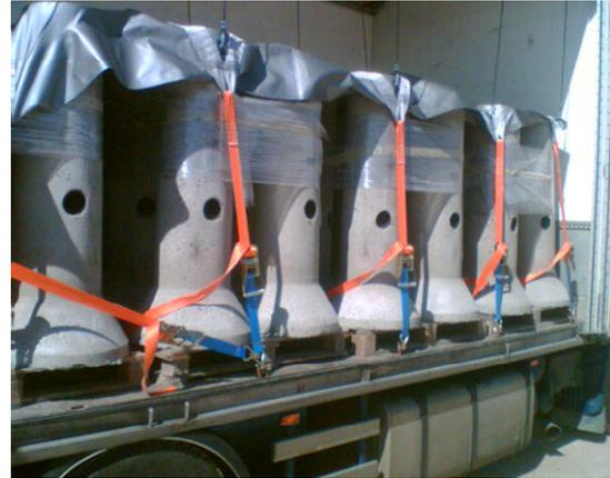
Surface pressure caused by tensioning is divided over entire surface and will therefore not damage the load. Sensitive load and soft packages cause no problem. Also, when high acceleration forces are applied, the load will not be damaged.
