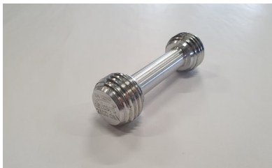
Ekeri tension roller/dumbbell Tension roller for Ekeri cargo securing system Also fits Bussbygg and Limetec Aluminium 50mm LC 25 kN
