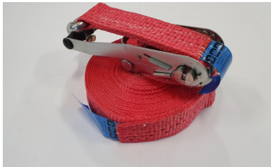
Cargo securing straps LC 2500 daN With standard 0,4m ratchet and hooks 50mm SHF 50 daN, STF 300 daN, LC 2500 daN Red, Orange and Blue
