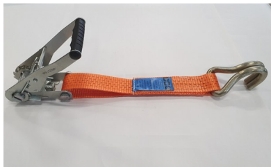
FIX ratchet 0,5 with d32mm J hook 0.5m Ratchet tensioner ends with wire J hook d32mm 50mm SHF 50 daN, STF 320 daN LC 2500 daN
