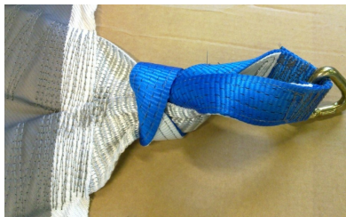
Short end with D-ring 50mm LC 2500 daN
